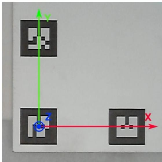
Figure 2.10: RoCKIn@Work Table reference frame example
