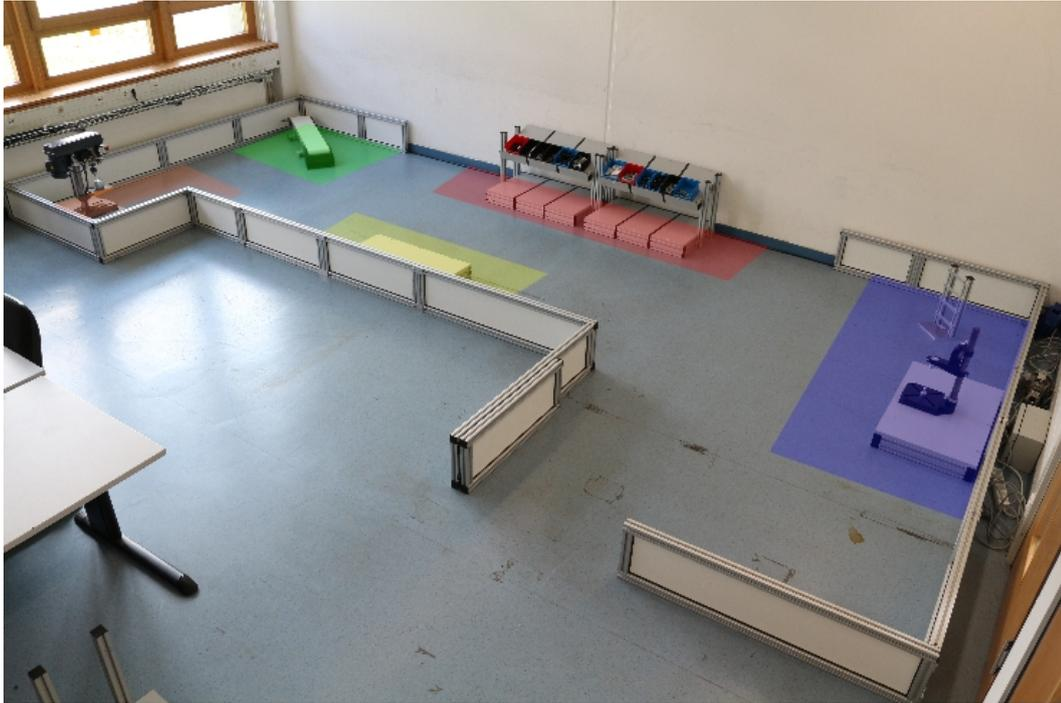
Figure 2.2: Example of the spatial areas in RoCKIn@Work environment. The spatial areas are shelves (red), force fitting workstation (blue), conveyor belt (green), drilling workstation (orange) and assembly workstation (yellow).
