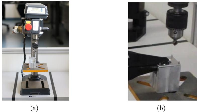
Figure 2.4: The RoCKIn@Work drilling machine (a) and a cover plate which is placed in the fixture of the drilling machine (b).
