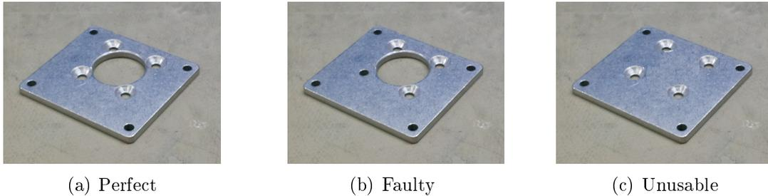
Figure 2.6: Three possible states of the cover plate
