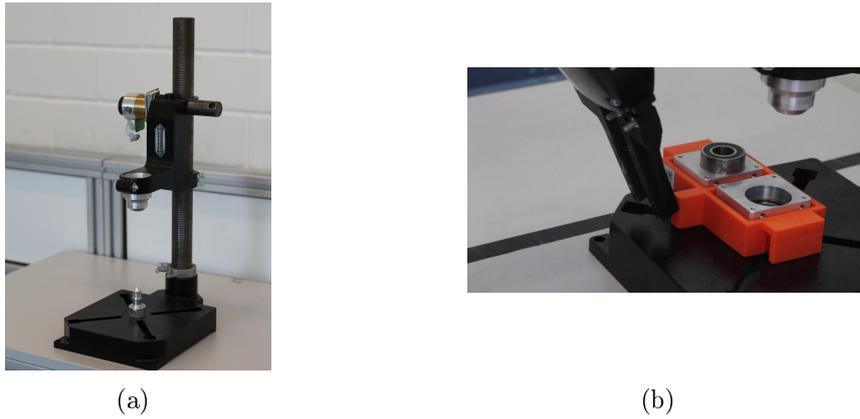
Figure 2.3: The RoCKIn@Work force fitting machine (a) and bearing boxes in the middle of force fitting process (b). The first bearing (right side) has been successfully force fitted into a bearing box.
