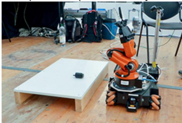
The robot has to identify the object in front of it, grasp and lift it and release it after a given time. The pose of the object in the gripper is not important, as long as the object is successfully grasped.
