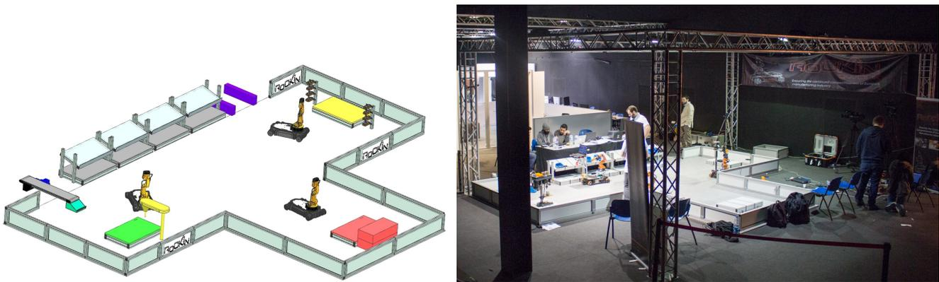
Figure 3 – RoCKIn@Work test bed, including the trusses for the MCS cameras on the right.
