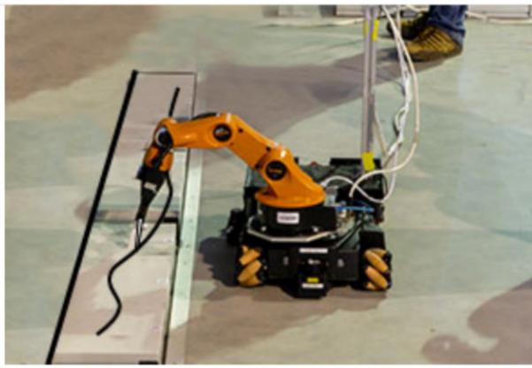
The robot has to follow a straight line/spline (without sensor feedback). Using a marker mounted on its end-effector an external system measures the path accuracy.
