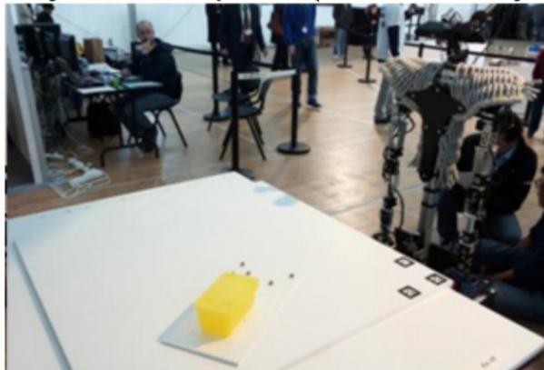
From a set of objects the robot has to detect, recognize and locate an object placed in front of it. Objects could be for example a coffee mug, a knife or a gold-colored picture frame.
