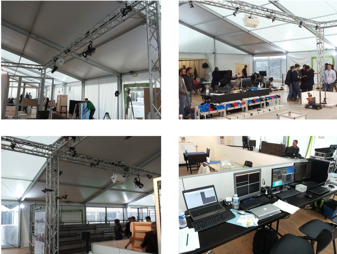
Figure 4.3: Four snapshots of the benchmarking system at Toulouse. Clockwise from top left: trusswork with cameras (and spotlights) above the RoCKIn@Home testbed; trusswork above the RoCKIn@Work testbed; some of the PCs used by the Benchmarking System; motion capture cameras used for FBM1.
