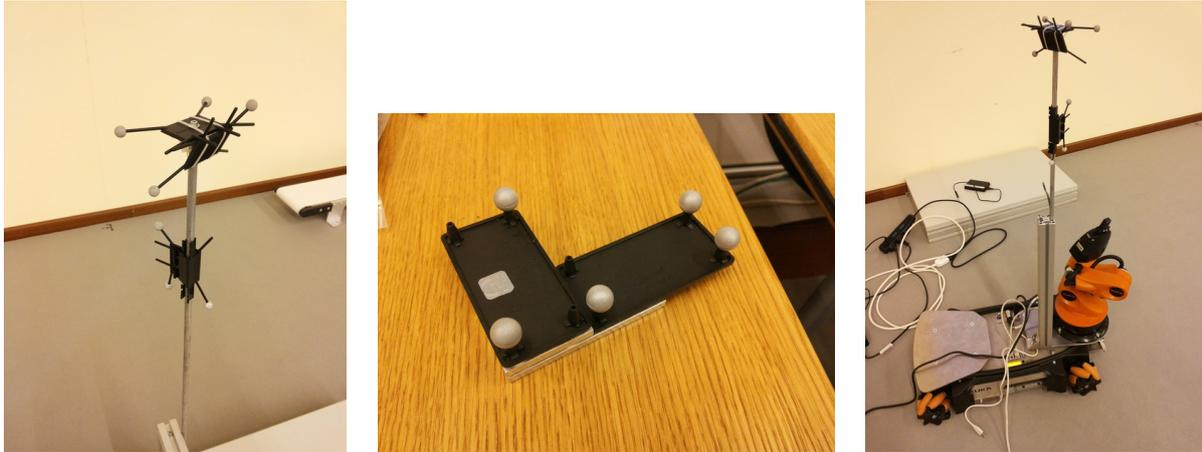
Figure 3.4: Two examples of rigid bodies fitted with markers, and a robot equipped with one of them.
