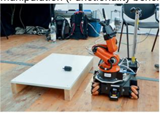
The robot has to identify the object in front of it, grasp and lift it and release it after a given time. The pose of the object in the gripper is not important, as long as the object is successfully grasped.
