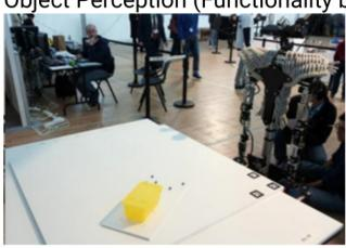
From a set of objects the robot has to detect, recognize and locate an object placed in front of it. Objects could be for example a tray, an axis or a bearing box.
