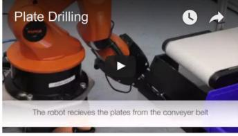
In this task the robot has to pick up a cover plate from a conveyor belt, conduct a quality check and perform one of three tasks according to the quality of the plate: perfect - collect; unusable - throw away; faulty - place inside drilling machine for rework.
